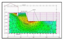
Fig. 10. Distribution of horizontal efforts in the ground next to the neighbouring building at the initial stage
