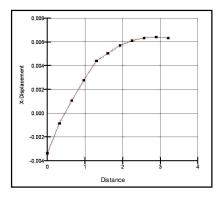
Fig. 13. The chart of horizontal displacement of the joint network points on the inner side of the wall
