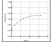
Fig. 11. The chart of horizontal displacements of the ground of the inner side of the wall
