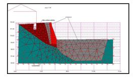
Fig. 9. Discretization of the bulk ground
