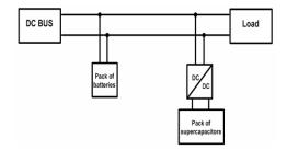
Fig. 5. General schema used for constant current charge method
