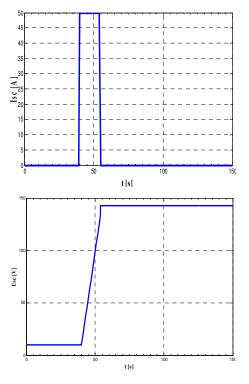
Fig. 9. Simulations characteristics obtained by the constant current (50 A) charge method for BPAK0058 E015 B1 module
