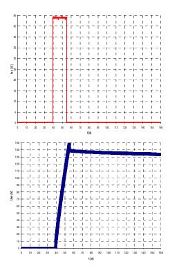
Fig. 8. Experimental characteristics obtained by the constant current (50 A) charge method for BPAK0058 E015 B1 module
