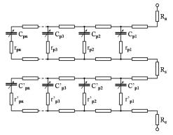
Fig. 1. The RC series model of a supercapacitor
