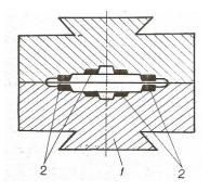
Fig. 1. Bimetallic mould: 1 - basic material; 2 - high alloyed material
