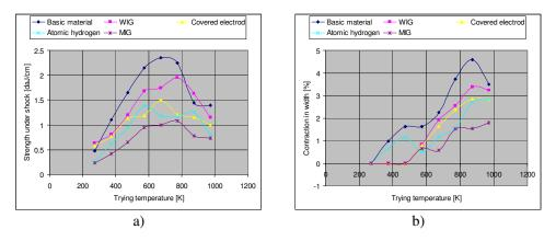
Fig. 2. Variation of mechanic properties obtained by bending trial through shock: a) variation strength under shock; b) variation contraction in width
