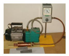
Fig. 3. *Laboratory vacuum sucking device*
