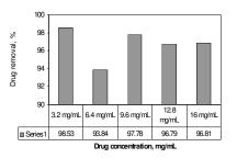
Fig. 2. Variation of streptomycin removal on Purolite anion exchanger
