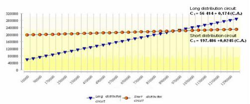
**Diagram 1.** Comparing the functions of the two distribution circuits
