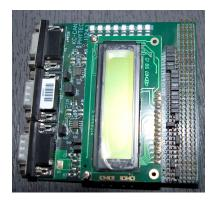
Fig. 7. Mini robot's CPU
