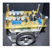
Fig. 5. The base with wheels for flexible mini robot
