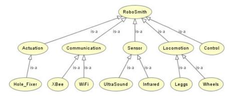
Fig. 11. Classes hierarchy for RoboSmith architecture
