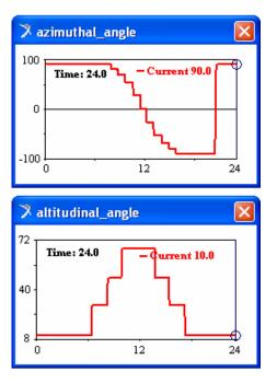
Fig. 8. The motion laws of the PV platform
