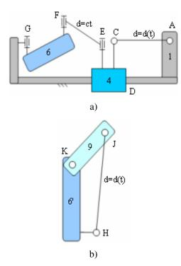
Fig. 4. The MBS model with minimum number of bodies
