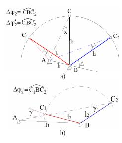
Fig. 3. *a*) Initial and final position of the linkage for minimum admitted  $\gamma$  and intermediary position for maximum  $\gamma$ ( $\gamma_{max} = x$ ) when  $l_1 < l_2$ ; *b*) Initial and final position of the linkage when  $l_1 > l_2$
