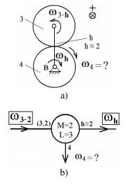
Fig. 4. a) Differential planetary gear pair and its b) black box scheme
