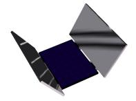
Fig. 1. Low solar concentrating system build up by a photovoltaic module and two lateral disposed mirrors
