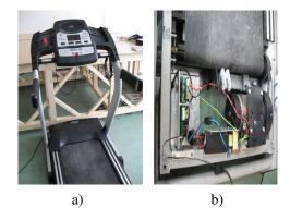
Fig. 2. Energetics Power Run 3000 HRC - structure (a) DC motor, control module (b)
