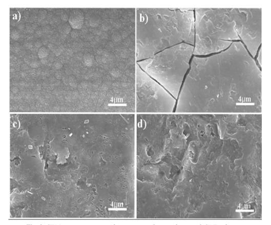
Fig. 2. SEM microstructures after reacting glass surfaces with SBF solution; (a) BG1, (b) BG2, (c) BG5, and (d) BG8.
