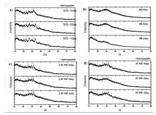
Fig. 1. XRD analysis after reaction in SBF solution of bioactive glasses (a) BG1, (b) BG2, (c) BG5, and (d) BG8.
