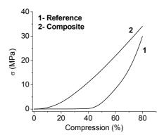
Fig. 6. Stress - compression strain of wood composite and reference in dry state
