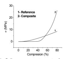
Fig. 7. Stress- compression strain of wood composite and reference in contact with 86% RH atmosphere
