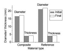
Fig. 5. Dimensional changes of composite and reference in 86% RH atmosphere
