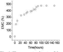
Fig. 4. Water sorption kinetic of the obtained composite
