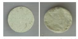
Fig. 2. Reference pressed wood flour (left) and obtained wood composite (right)
