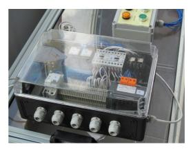
Fig. 3. Electrical module for independent command of conveyor belt engine of flexible line FMS 200
