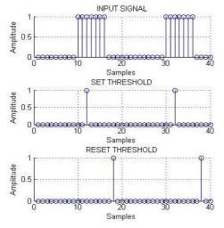
Fig. 4. Implementation results of Bistabil function on a sampled input signal, active on the landing
