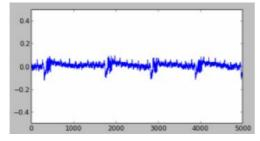
Fig. 2. USB power line noise
