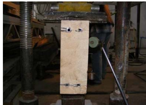
Fig. 4. Cross section of double reinforced beam with RMP
