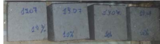
Fig. 1. Cubic specimens in climatic room
