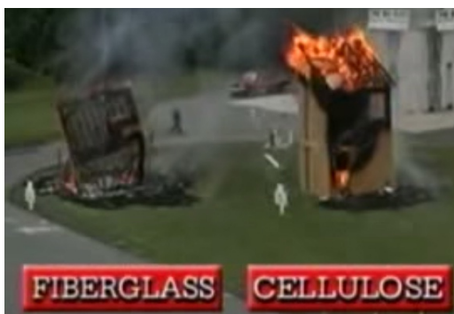
Fig. 8. Reaction to fire – Comparison cellulose vs. Fiber glass wool
