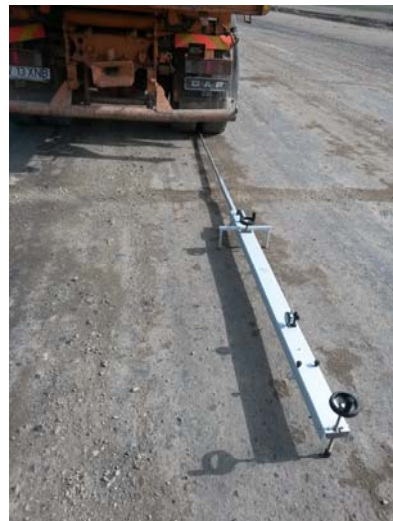
Fig. 1. Benkelman beam test
