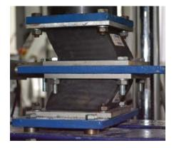
Fig. 11. The elastomeric bearing displacement
