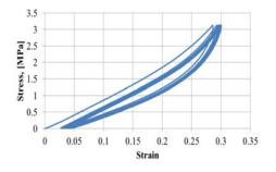
Fig. 4. The stress-strain curves of CR
