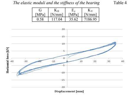
Fig. 12. The force-displacement curves of elastomeric bearings
