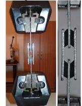
Fig. 8. The shear test of elastomer [7]
