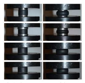
Fig. 3. The compression test of elastomers
