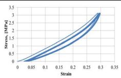
Fig. 5. The stress-strain curves of NR
