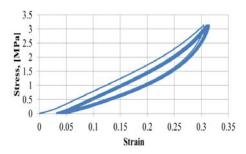
Fig. 7. The stress-strain curves of SBR
