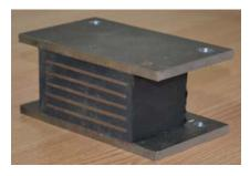
Fig. 10. The elastomeric bearing
