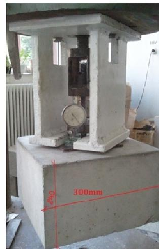
Fig.4. Developed tension test rig for confined tests
