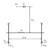
Fig. 3. The mass loads on the wagon wheels
