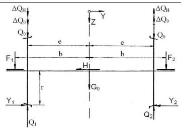
Fig. 1. The vehicle axle mass load transfers
