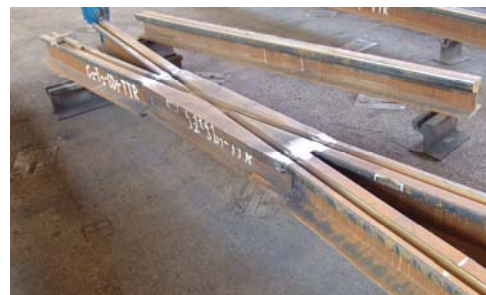
Fig.10. Tramway frog ready for montage
