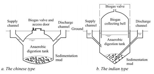
Fig. 6 Types of rural biogas reactors
