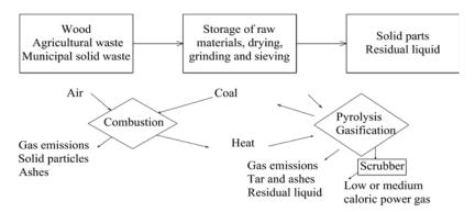
Fig. 3 Combustion processes diagram
