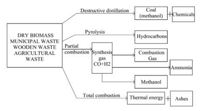
Fig. 1 Dry biomass conversion technologies
