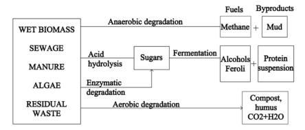
Fig. 2 Wet biomass conversion technologies
