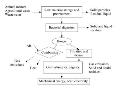
Fig. 5 Diagram of anaerobic digestion process
