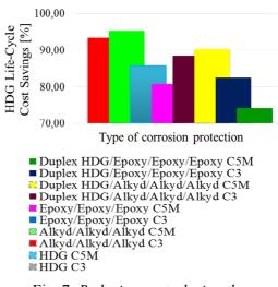
Fig. 7. Reducing costs during the lifetime of the considered systems when using corrosion protection by galvanizing HDG
