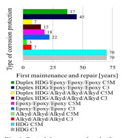
Fig. 4. Period that occurs after the first intervention of maintenance and repair
