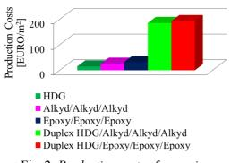
Fig. 2. Production costs of corrosion protection
