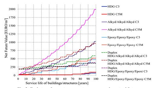
Fig. 3. Evolution of corrosion protection costs over the entire lifetime
