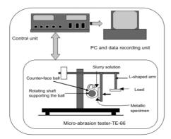
Fig. 2. Mechanism of microabrasion [17]
