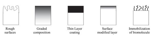
Fig. 1. Metallic material surface modification techniques [8]
