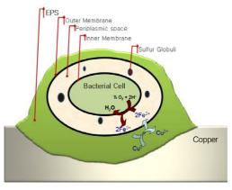
Fig. 4. Biomachining mechanism [12]
