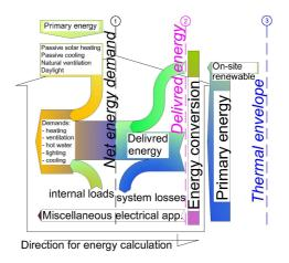
Fig. 3. Primary energy calculation limits
