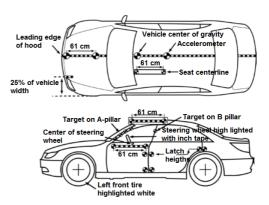
Fig. 13. Crash markings on the vehicle
