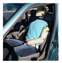
Fig. 17. Custom built crash test dummy
