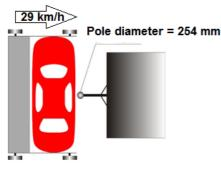
Fig. 4. *Side impact with a pole*
