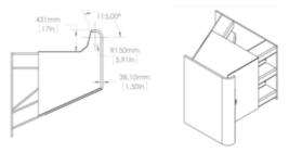
Fig. 12. Dimensions of the barrier
