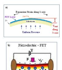
Fig. 10. a) A PZT layer having the substrate, the top and base electrodes indicated;
