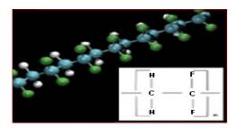
Fig. 3. *PVDF is a high-molecular weight* polymer with repeat unit  $[CH_2-CF_2]$
