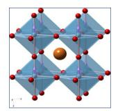
Fig. 1. Atomic structure - Barium Titanate
