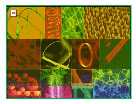
Fig. 9. ZnO nanostructures (nanocombs, nanorings, nanohelixes/nanosprings, nanobows, nanobelts, nanowires, nanocages)
