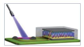
Fig. 17. A ZnO based UV nanosensor coupled with a nanogenerator in an energetic independent nanosystem
