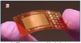
*b) The experimental built device* Fig. 13. *A totally encapsulated nanogenerator*
