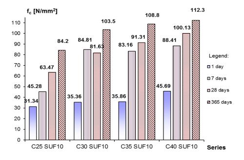
Fig. 3. Compressive strengths
