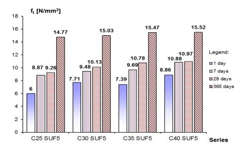
Fig.2. Bending tensile strengths
