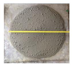
Fig. 7. Spread after preparation
