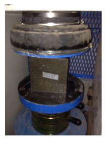
Fig. 11. Compression Strength determination
