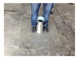
Fig. 3. The cone spread equipment
