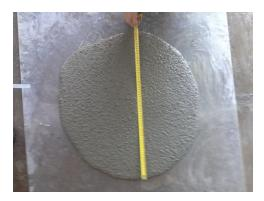
Fig. 4. The Spread Test
