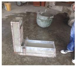
Fig. 6. The L box test
