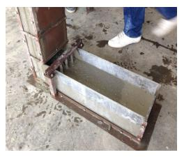
Fig. 8. L box after preparation
