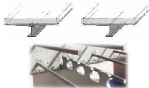
Fig. 5. VFT ® solution for composite bridges
