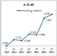
Fig. 1. Swelling values in time for asphalt base concrete with crushed gravel, designed for road pavements with light traffic A.31.nb
