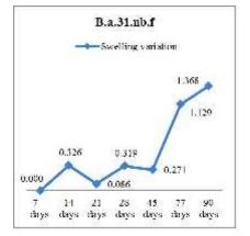
Fig. 2. Swelling values in time for asphalt concrete with crushed gravel for the binder layer B.a.31.nb.f
