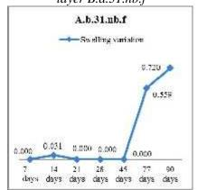
Fig. 3. Swelling values in time for the asphalt base concrete for bituminous base course A.b.31.nb.f
