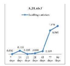
Fig. 4. Swelling values in time for asphalt base designed for light traffic A.31.nb.f
