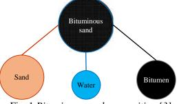
Fig. 1 Bituminous sand composition [3]
