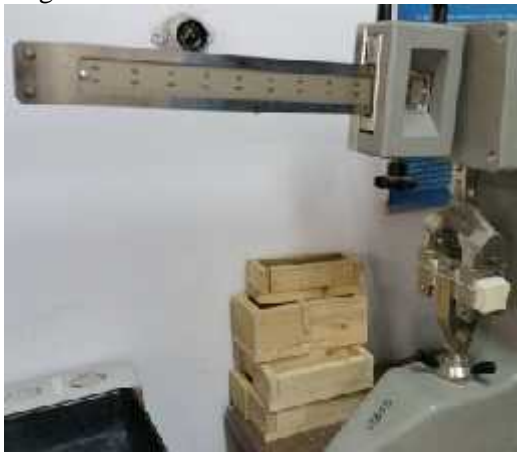
Fig. 2 The machine used for the determination of flexural tensile strength, the Building Materials Laboratory of the Faculty of Civil Engineering
