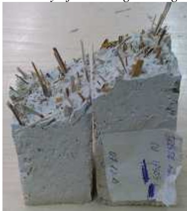
Fig. 3 The prism ends of a 40x40x160 mm test sample resulted from the flexural tensile strength test.
