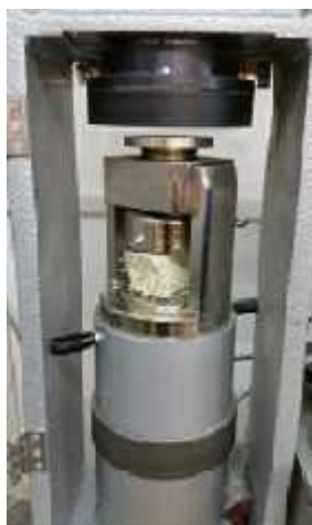
Fig. 5a Compression test for mortar A2
