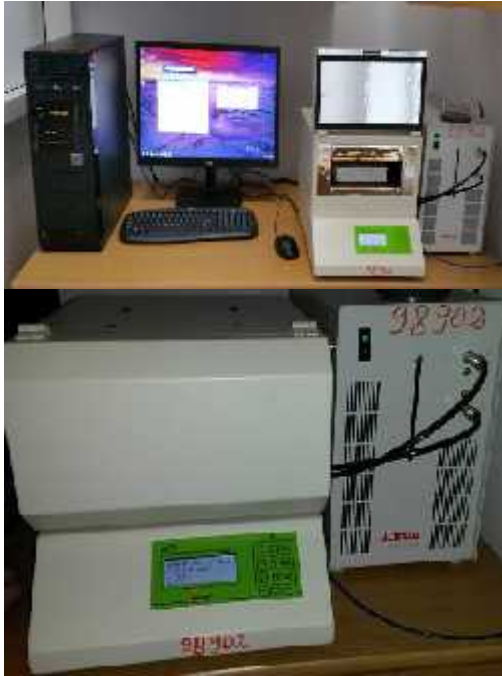
Fig. 6 The thermal conductivity measuring instrument
