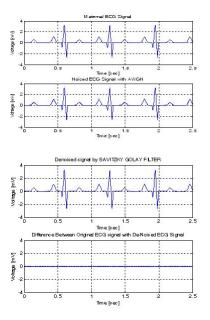
Fig 6. Maternal electrocardiogram ECG signal (Savitzky and Golay Filter SNR=40 dB (Low) as a cubic filter to information frames of length 41(k=3, f=41))
