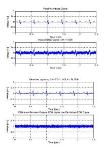
**Fig 7.** Fetal electrocardiogram ECG signal (Savitzky and Golay Filter SNR=0 dB (High) as a cubic filter to information frames of length 41(k=3, f=41))
