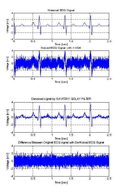
Fig 5. Maternal electrocardiogram ECG signal (Savitzky and Golay Filter SNR=0 dB (High) as a cubic filter to information frames of length 41(k=3, f=41))
