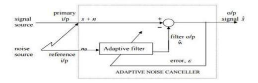
Fig 4. Basic Structure of an Adaptive noise cancellation
