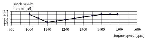
Fig. 5. Smoke emission versus speed
