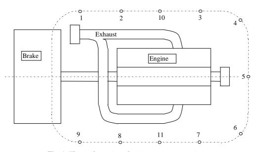
Fig. 4. The configuration of noise measurement points
