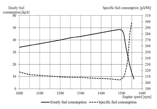
Fig. 2. Hourly and specific fuel consumption versus speed
