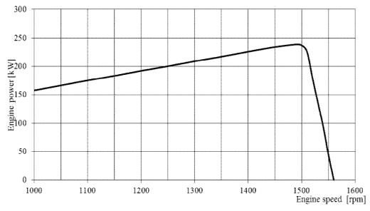
Fig. 1. Full load speed characteristic
