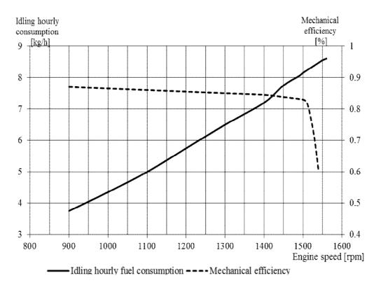
Fig. 3. Mechanical efficiency and idling hourly fuel consumption versus speed
