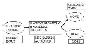
Fig. 5. Schematic function of an actuator
