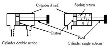
Fig. 7. Cylinders hydraulic/pneumatic
