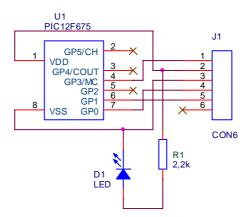
Fig. 2. Electrical schematic programmer
