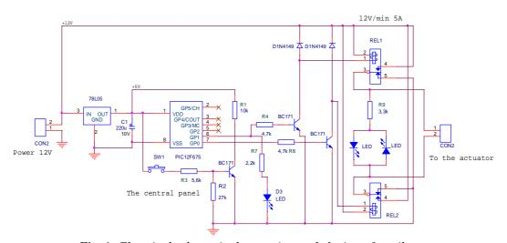
Fig. 1. Electrical schematic the opening and closing of a tailgate
