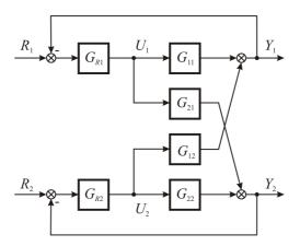
Fig. 1. Multi-input-multi-output control system
