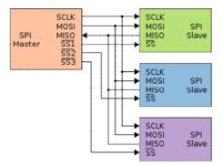
Fig. 4. Serial Peripheral Interface
