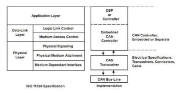
Fig. 1. The layered ISO 11898 architecture
