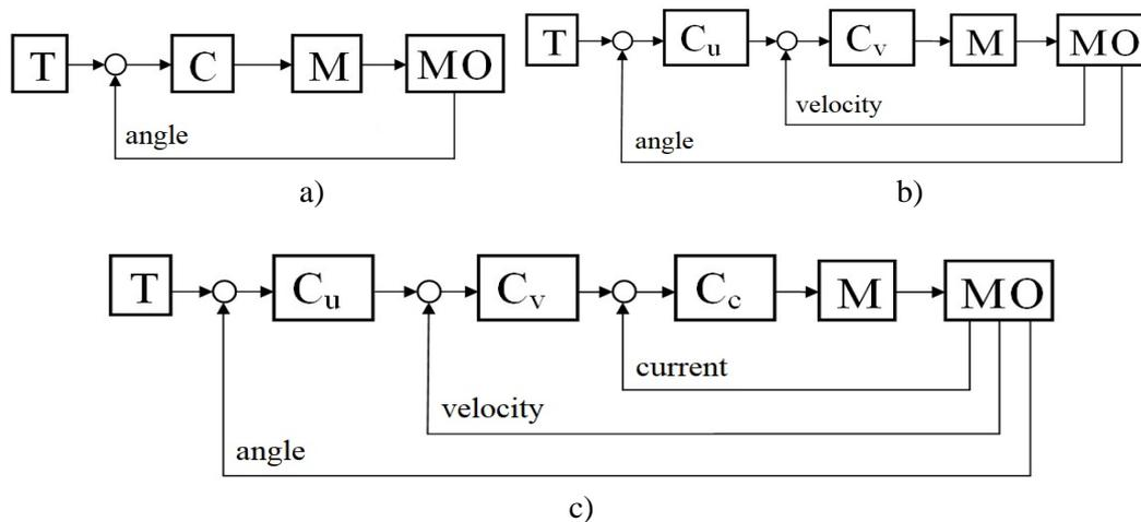
Fig. 2. *Single-loop (a), two-loop (b) and three-loop (c) control schemes*
