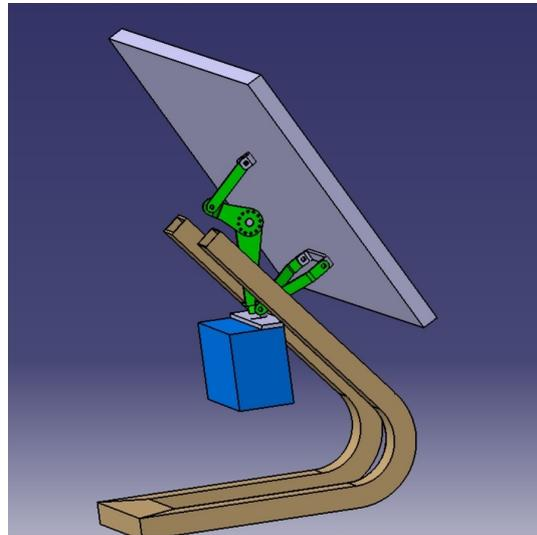
Fig. 3. The virtual prototype of the dual-axis sun tracking mechanism
