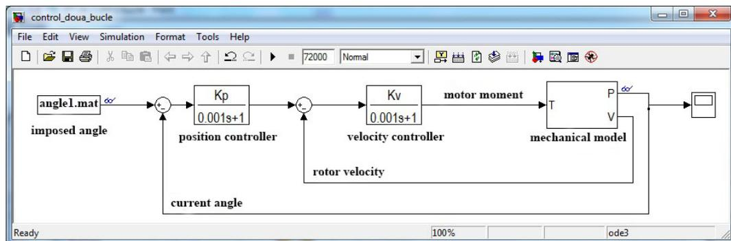
Fig. 8. *The two loop in cascade control system model*
