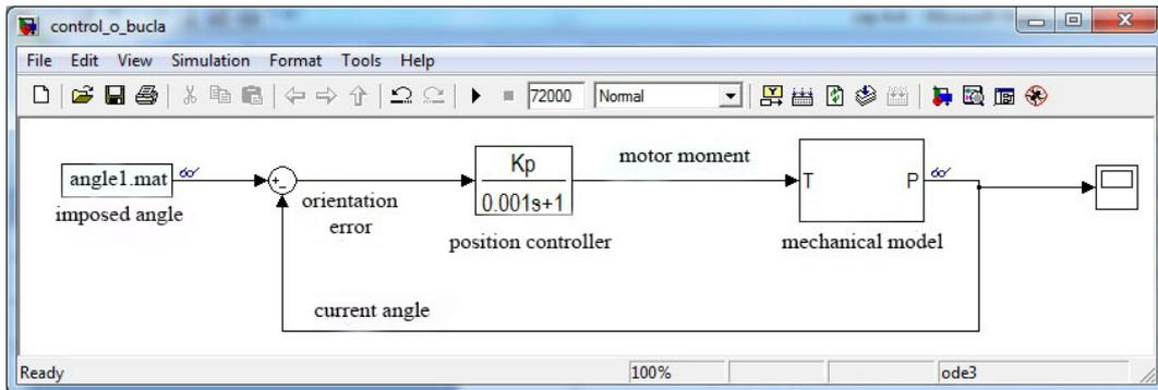
Fig. 6. Single loop control system model
