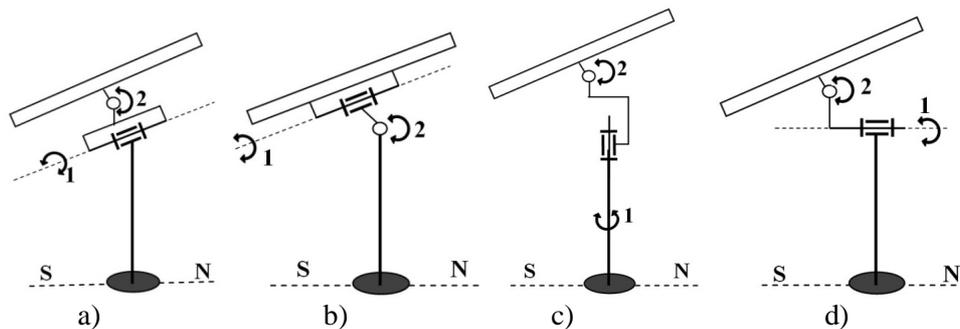
Fig. 1. *Dual-axis solar trackers* [4]
