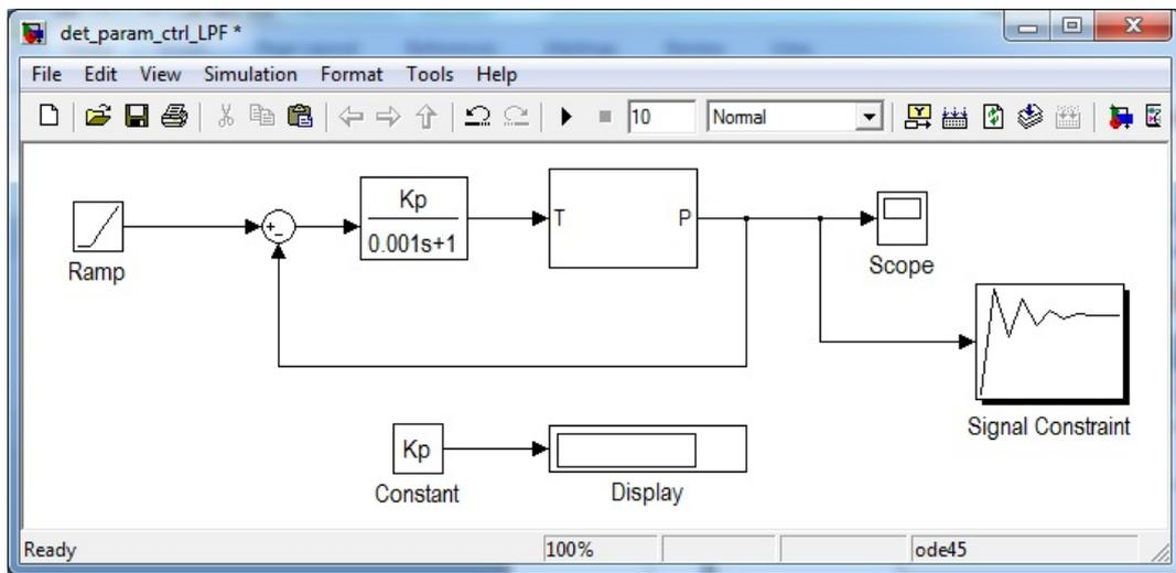
Fig. 5. The control system for determining the parameters of the controller
