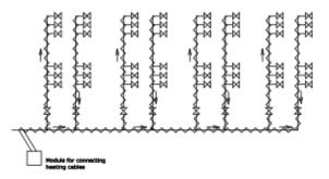
Fig.3. The scheme of the heat loss compensation with electrical heated cables
