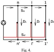
The unit equivalent resistance of the bar (s0iechiv) that's equal with 2L results from the equivalent of the corresponding load losses Dtotal i and Dcirc i.
