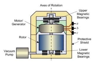
Fig. 2. Structure of a conventional flywheel [5]
