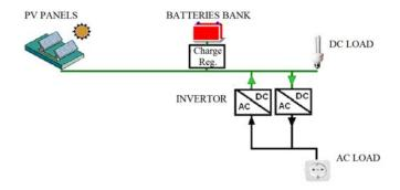
Fig. 5. Schematic diagram of the solar PV system [3]
