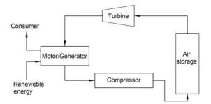
Fig. 3. Compressed air energy storage system
