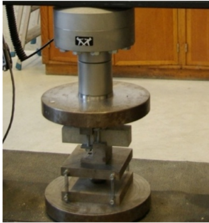
Fig. 2. Direct shear test
