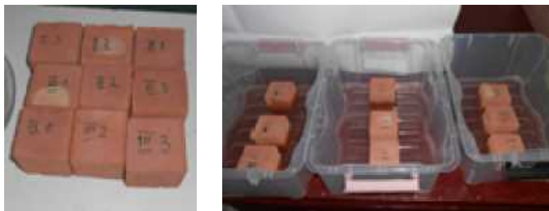
Fig. 1. (a) ceramic test samples; (b) ceramic test samples prepared to be immersed in sodium chloride solution
