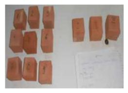
Fig. 1. Array-samples extracted from masonry ceramic elements
