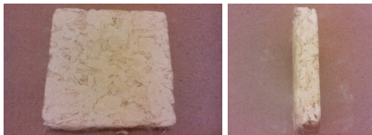
Fig. 2. Sample of wool bonded with hydrated lime, dimensions 150x150x30 mm
