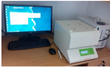
Fig. 4. Measuring device for thermal properties, Fox200
