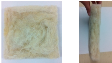
Fig. 3. Sample of wool bonded with adhesive, dimensions 200x200x30 mm
