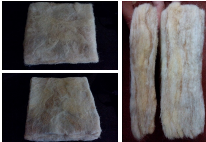
Fig. 1. Samples of wool without binder, dimensions 150x150 mm
