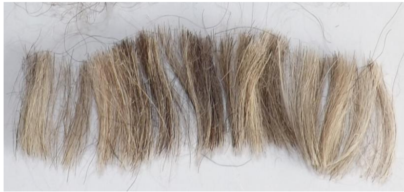
Fig. 1. Sheep wool fibers of 2-3 cm length, used in concrete composition
