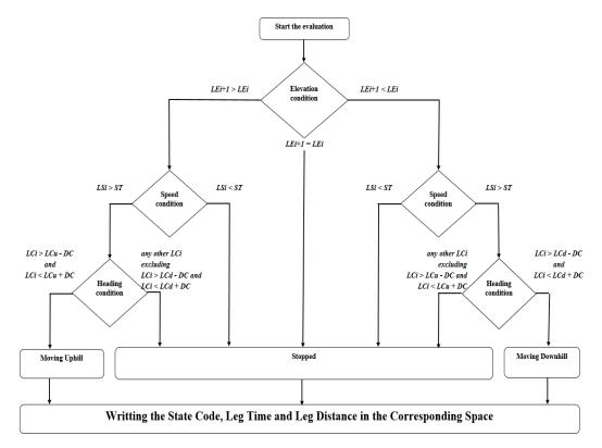
Fig. 3. Logic of the algorithm developed in Visual Basic for Applications ® under MS Excel ® to extract time consumption elements from the GPS data files
