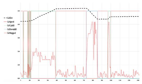
Fig. 4. A snapshot showing the carriage behaviour as interpreted by the algorithm against the variations in elevation and speed from the GPS data. Legend: red - stopped, green - uphill movement, blue - downhill movement, dotted red - leg speed, dotted black leg elevation (divided by a factor of 200)
