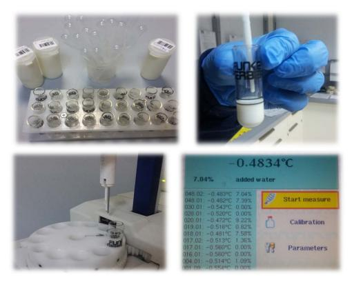
Fig. 4. The equipment used to establish the cryoscopic point of cow milk
