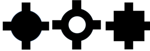
Fig. 3. Masks which were used for Hall Sensors Simulations. The image should be in black/white format to be accepted by the simulator (during simulation the black regions will represent the magnetic material)
